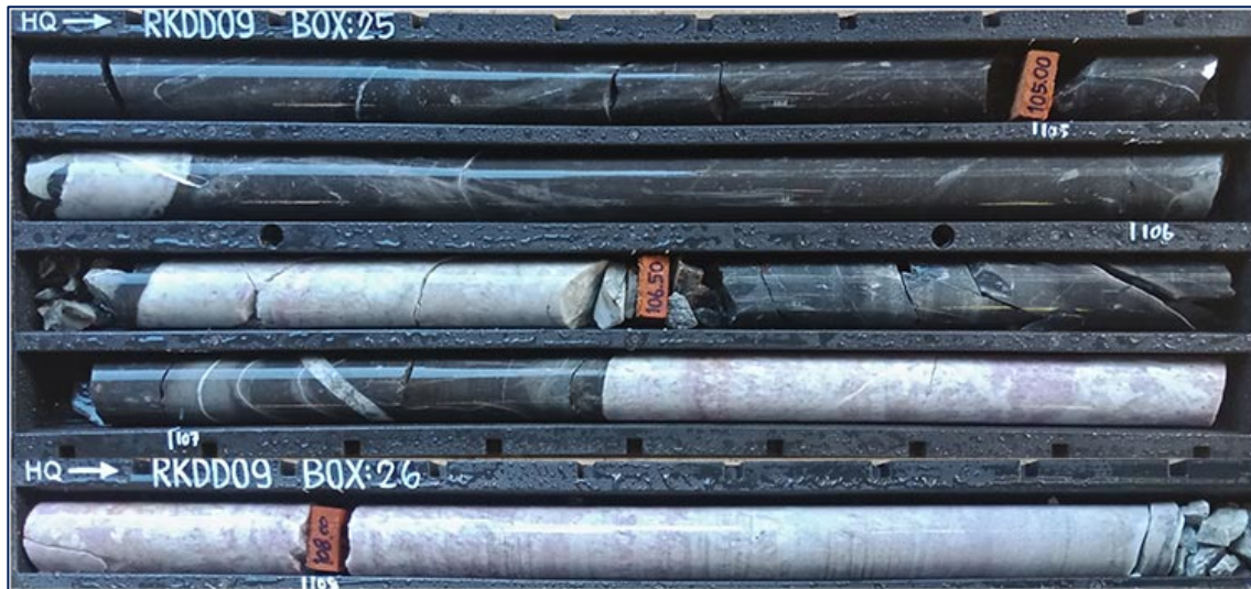
Photo 2: RKDD009 drill core from 104.2m to 108.7m, showing lepidolite pegmatite dykes (purple colours)
