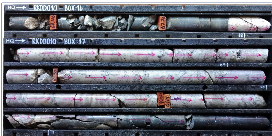
Photo 3: RKDD010-drill core from 67.3m to 71.8m, showing lepidolite pegmatite dyke (purple colours)
