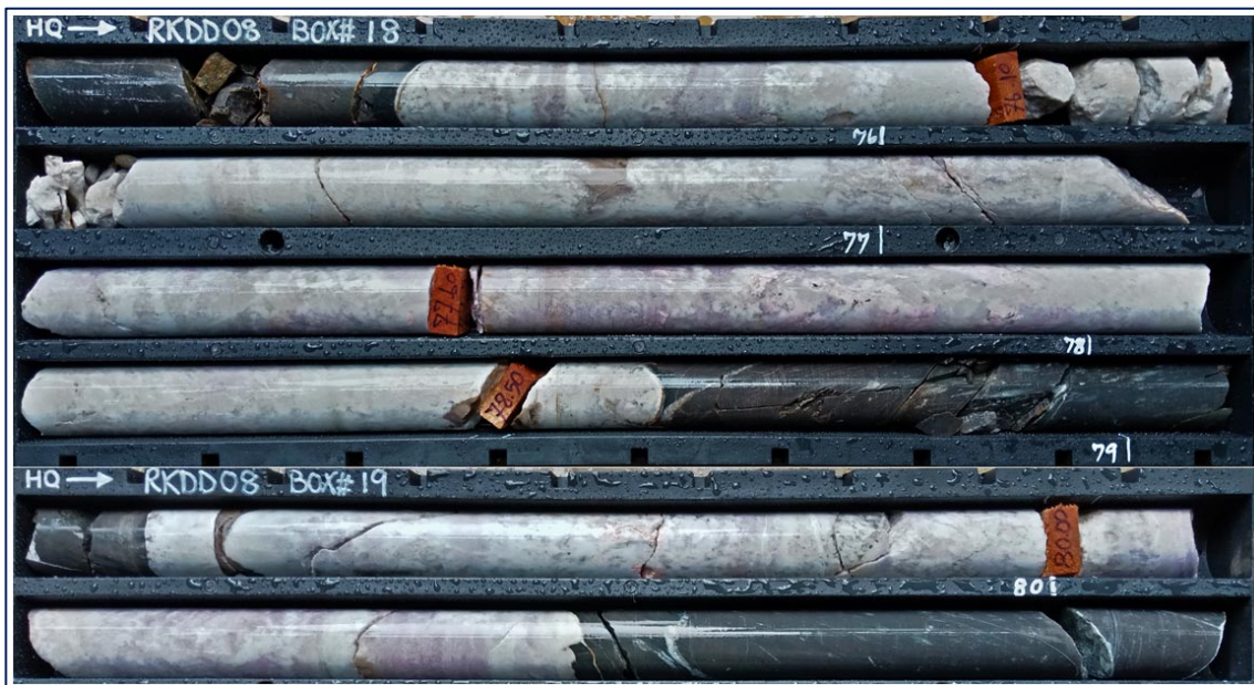
Photo 1: RKDD008-drill core from 75.3m to 81m, showing lepidolite pegmatite dyke swarm (purple colours)
